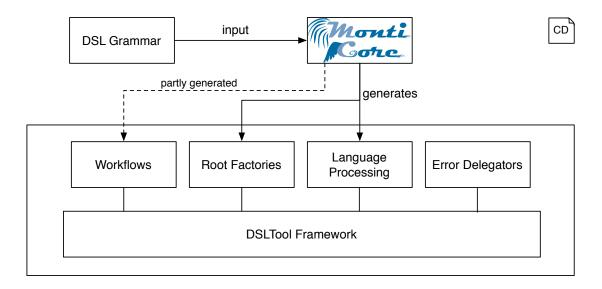
Figure 2.6: The basic architecture of a compiler developed with MontiCore [Kra09].
