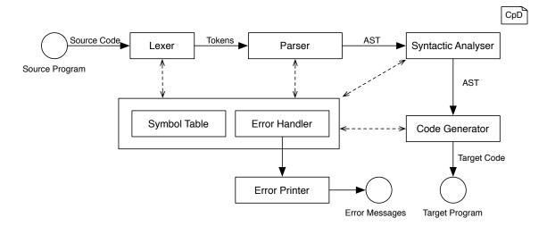
Figure 2.3: The basic architecture of a compiler. Circles denote inputs or outputs of the compiler, the boxes its components. Arrows denote the dataflow inside the compiler and their labels state, what data is transferred. The dashed arrows show other communication between components. [Mül08]
