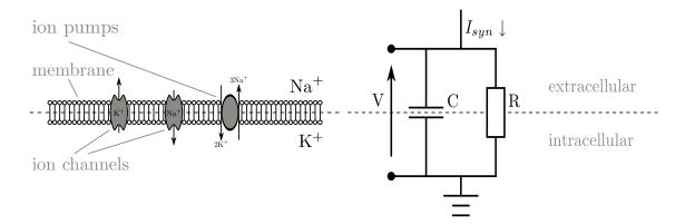
Figure 6.1: On the left a cross section of membrane and on the left the corresponding electrical circuit [Epp10].
